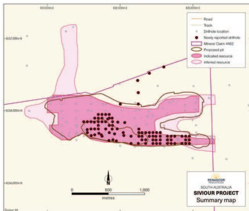
**Figure 2. Siviour Graphite Project, showing recently drilled holes in relation to previously drilled holes, Indicated and Inferred Resource outline and proposed pit design**
