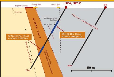
Sampling and mapping has defined extensive area of elevated copper and cobalt
