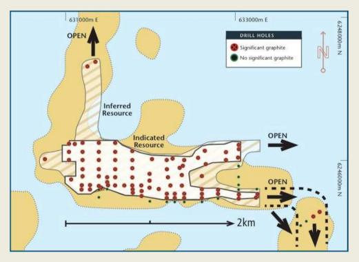
Siviour Indicated and Inferred Resource over outline of airborne electromagnetic conductivity anomaly
