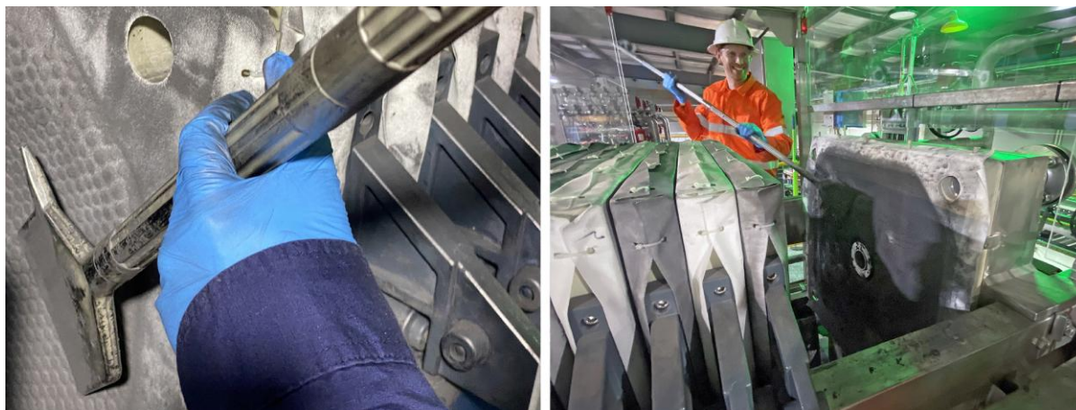
Figure 2. Operation of filter press at at Renascor's PSG demonstration facility in Adelaide
