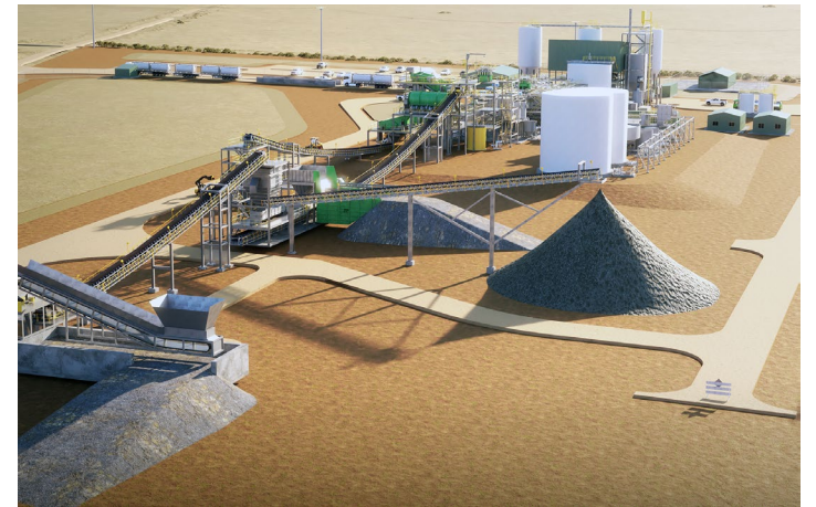
Conceptual illustrations of the maturing engineering design for the upstream operations at Arno Bay
